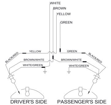
Note: Original inventory of the wiring kits were received with red/green/white wiring. The newer inventory has the standard black/brown/white wiring.
